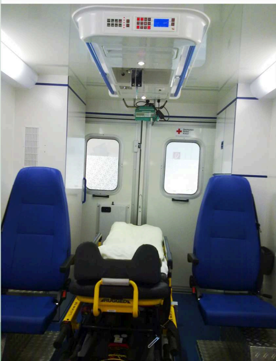
M1 getestete Betreuersitze in drehbarer Ausführung M1-tested side panel seats in swivelling execution
